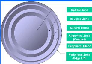
Fig. 2 – ESA ortho-6<sup>®</sup> lens. Hexa-curve reverse geometry, IT Patent 2002 Antonio Calossi. Material: Boston XO<sup>®</sup>, siloxy-fluoro-methacrylate, Dk 100 x 10<sup>-11</sup>
